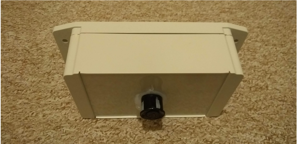
FIGURE 4.11: Sealed Sensor Node
