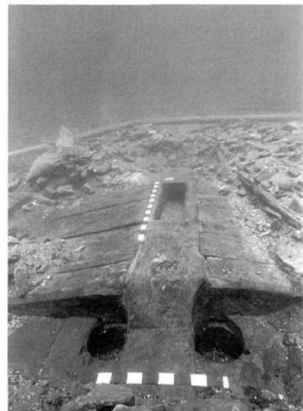
Figure 4.25(Above) The mast step-keelson structure of the 29M (James Ringer, 2007: I-209)
