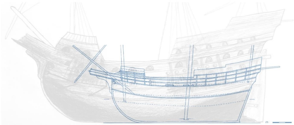
Figure 5.3 Reconstruction of the Santiago de Galicia galleon, (Drawing by the author at the background) as against the reconstruction of the complete hull of the 24M vessel (In blue), considered a nao, made by Parks Canada. Both reconstructions are made at the same scale and following their proportions. This was one of the possibilities the upperworks of the 24M could have been built like (Grenier et alii, 2007: III-220).
