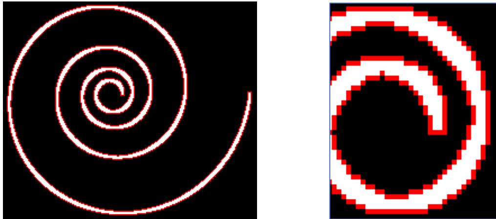
Figure 2-2: Moore's Boundary algorithm. Left: the binary image with Moore's algorithm applied. Right: A close up of spiral centre showing 8-connectivity.
