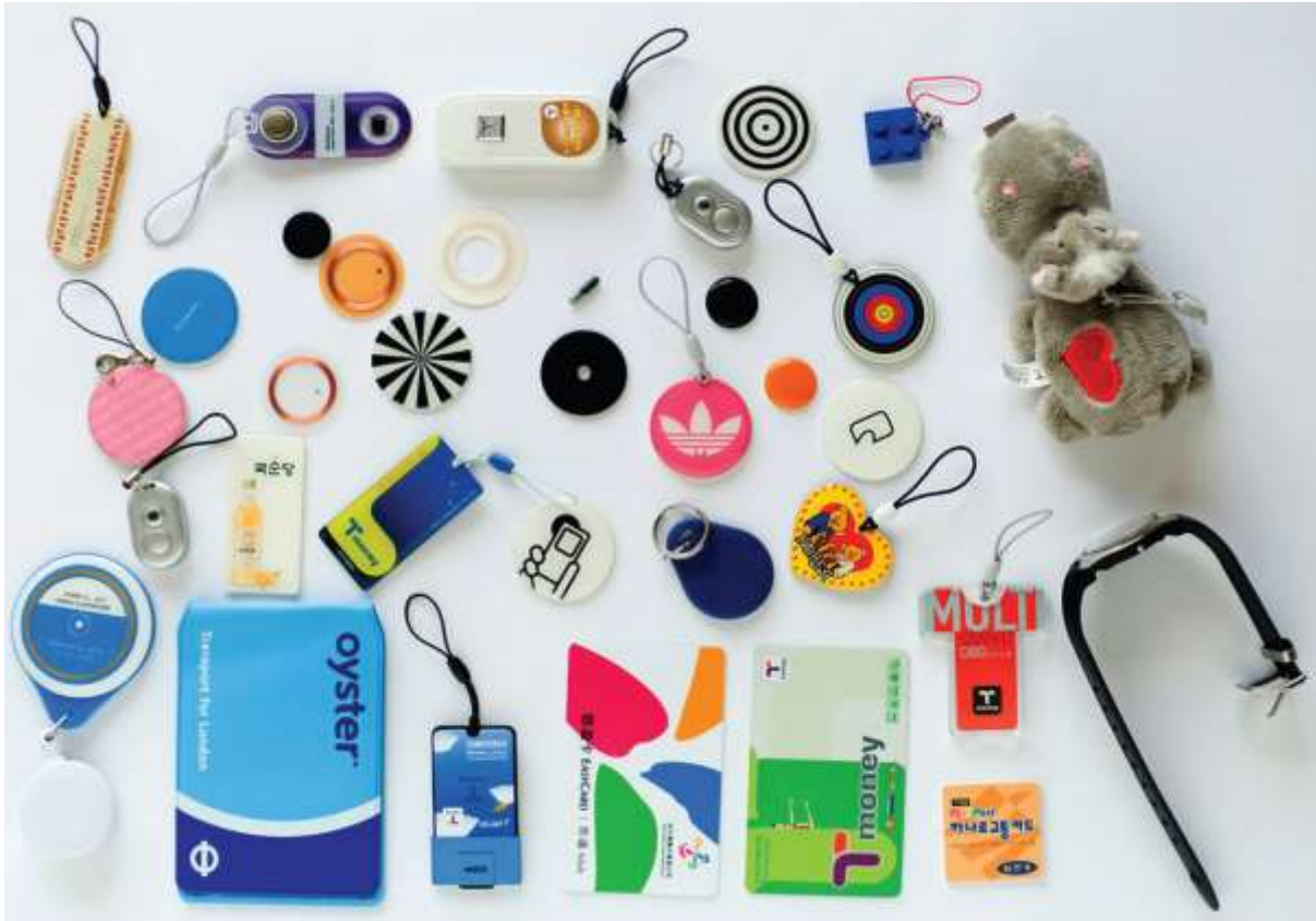
Figure 2.9: RFID tags come in different shapes and sizes (Source: Arnall 2007).
