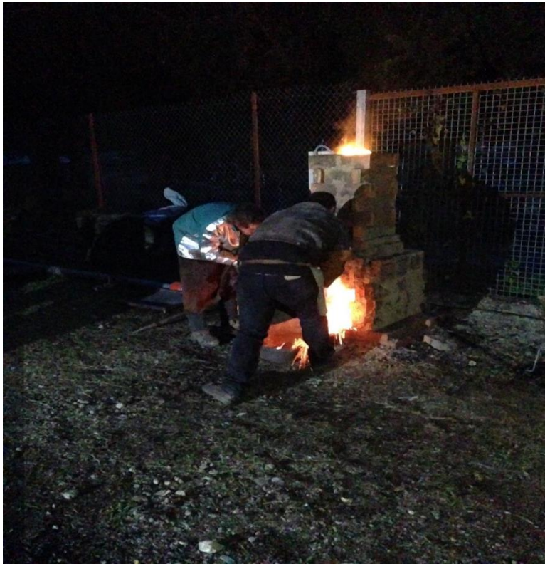
Figure 3.10 Removal of the bloom from the furnace, during the metalworking fair at Arles-Sur-Tech (source: S. Jenkins Carter).
