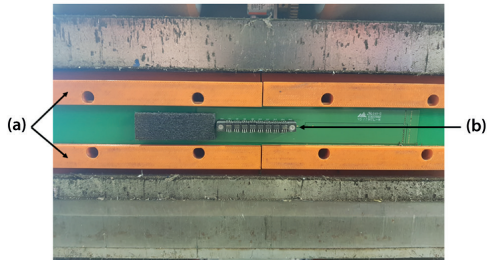
Figure 3. The sensor array in a 3D printed housing designed to give a lift-off of 0.5 mm, where: (a) is the 3D printed housing; and (b) is the array of eight 5 mV/G Hall-effect sensors
