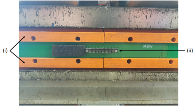
Figure 3.15: Showing the sensor array in a 3D printed housing to give a lift-off of 0.5mm where; (i) is the 3D printed housing and (ii) is the array of eight 5mV/G Hall effect sensors.
