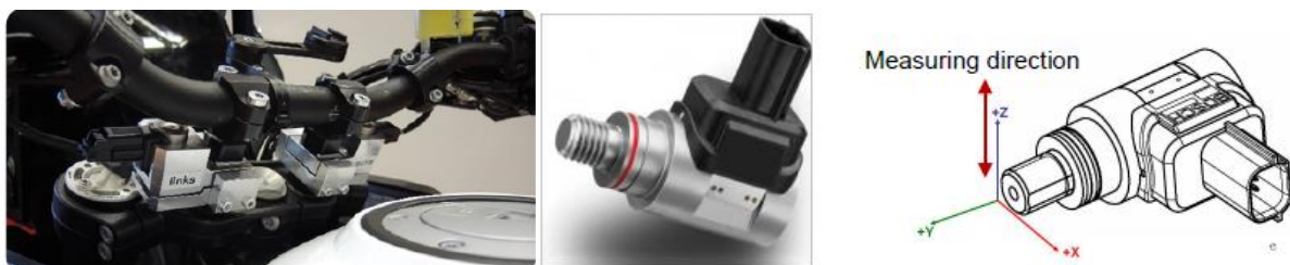
Figure 69: Force Measuring Bolts employed for Steering Torque Measurement (Wahl Et Al. 2020)
