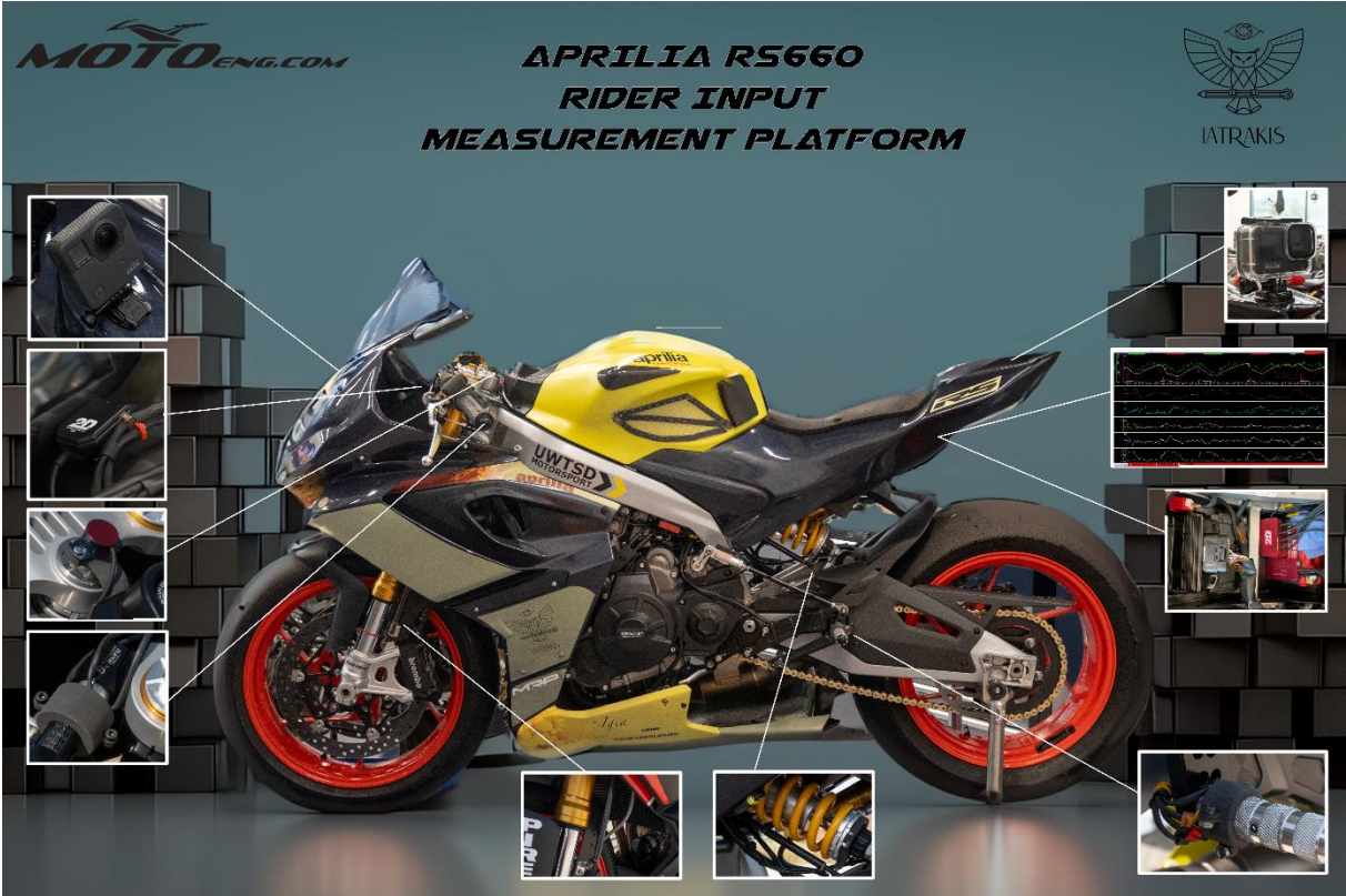
Figure 6: The RS660 Rider Input Measurement Platform along with the aftermarket and custom sensors.
