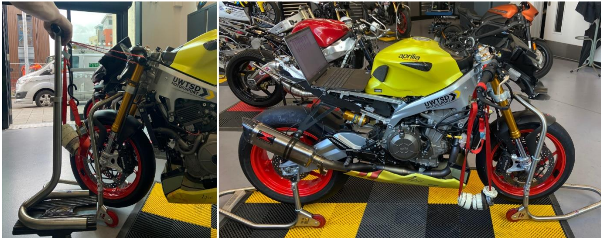
Figure 16: Handlebar Calibration using weights - X-axis (Left) - Y axis (Right).
