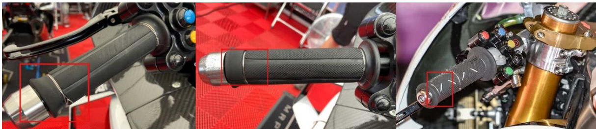
Figure 14: Wear on outer area of handlebar grips. Champion Alpha Van Zon IDM SBK Team (Left & Right) - Honda HRC MotoGP (Right)
