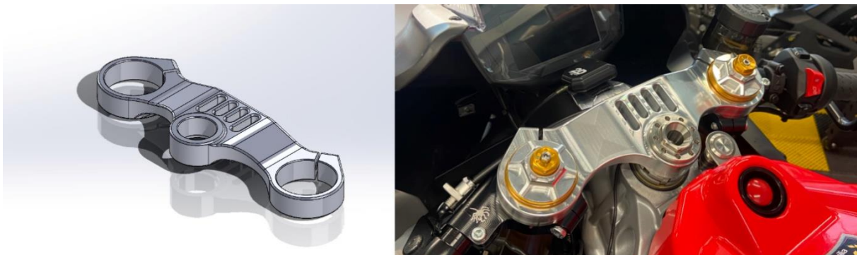
Figure 7: CAD Drawing to Finished Top Clamp.
