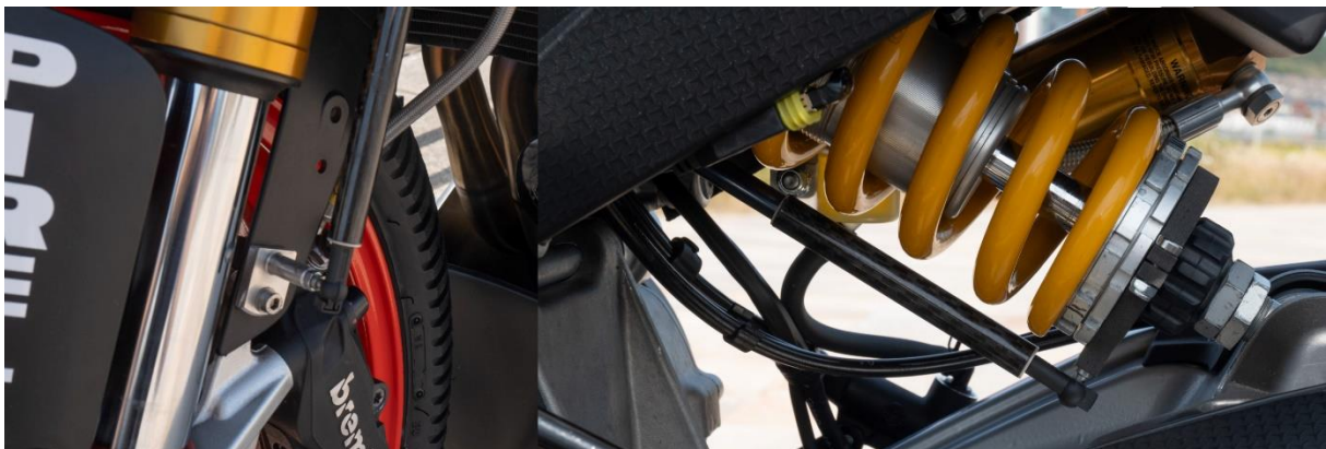
Figure 5: Suspension Position Potentiometers Mounted on the Aprilia RS660.
