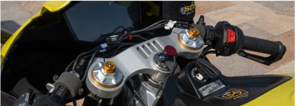
Figure 10: View of the motorcycle cockpit as in use, with strain gauges and wiring protected and sealed.
