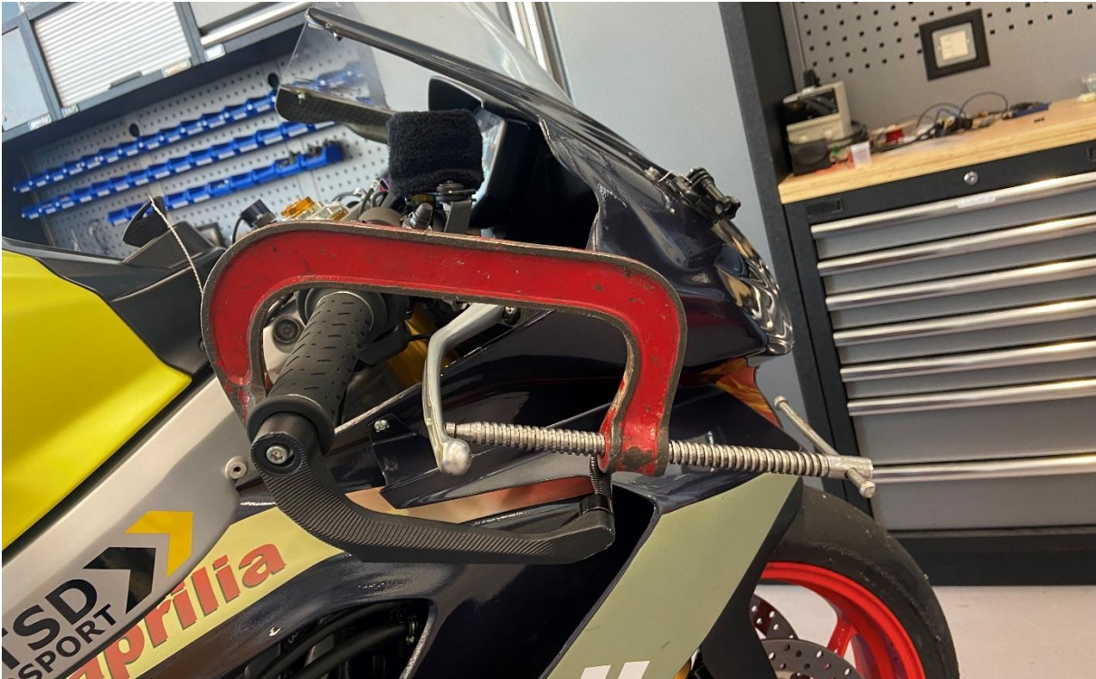
Figure 18: Validating strain measured by pulling force on levers.
