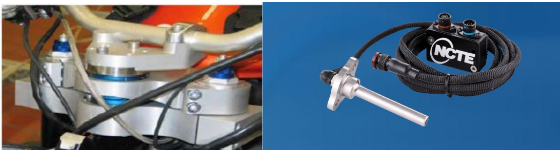
Figure 68: Steering Torque Measurement. (Wahl et al. 2020) (Left) – NCTE Internal Torque Measurement Sensor. (NCTE 2023) (Right)
