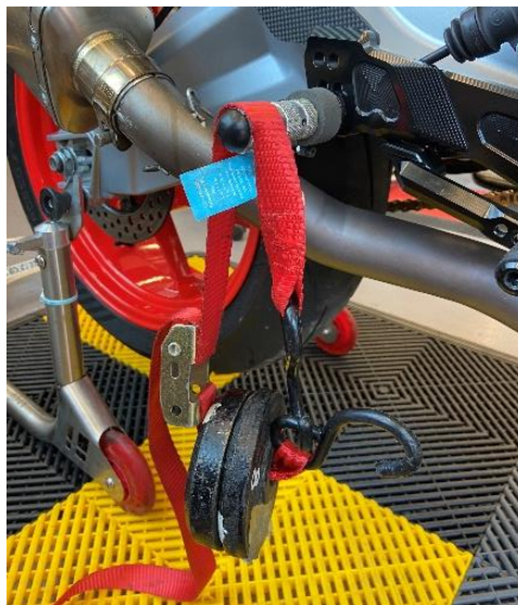
Figure 22: Footpeg Calibration Weight loading.
