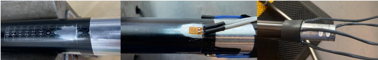
Figure 9: Prepared area (left) - Bonded and Soldered Strain Gauge (Middle) – Strain Gauges Sealed and Wires Heat shrunk (Right).
