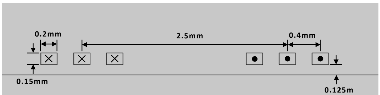
Figure 3.17: Simulated Design of MLC at 0mm Lift-off
