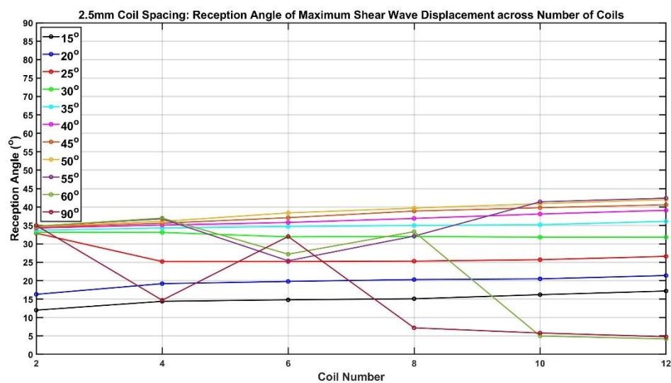
Figure 6.26: Graph of Shear Wave Reception Angle across Number of Coils for 2.5mm Coil Spacing
