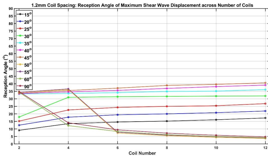
Figure 6.47: Graph of Shear Wave Reception Angle across Number of Coils for 1.2mm Coil Spacing
