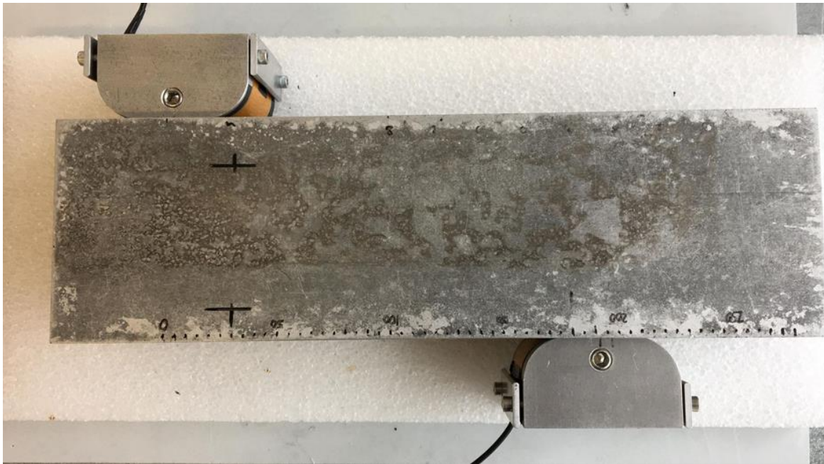
Figure 4.78: EMAT Beam Steerability Experimental Setup
