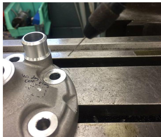
Figure 13 - Drilling of Pressure Passageway (GTPE, 2019)
