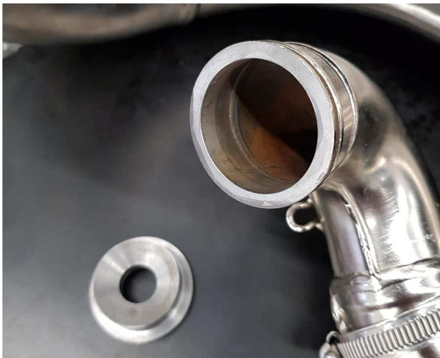
Figure 2 - Exhaust Port Restrictor Adjacent to Modified Exhaust
