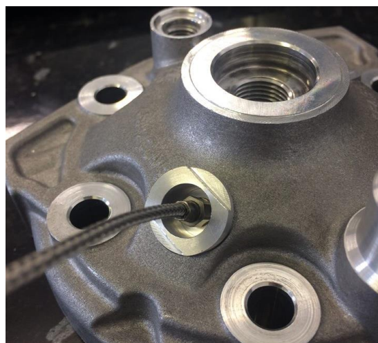
Figure 19 - Pressure Sensor and Insert in Head
