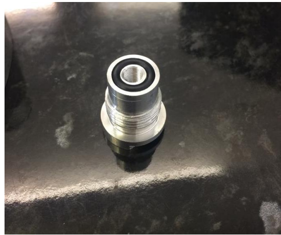
Figure 15 - Machined Insert and O-ring (GTPE, 2019)
