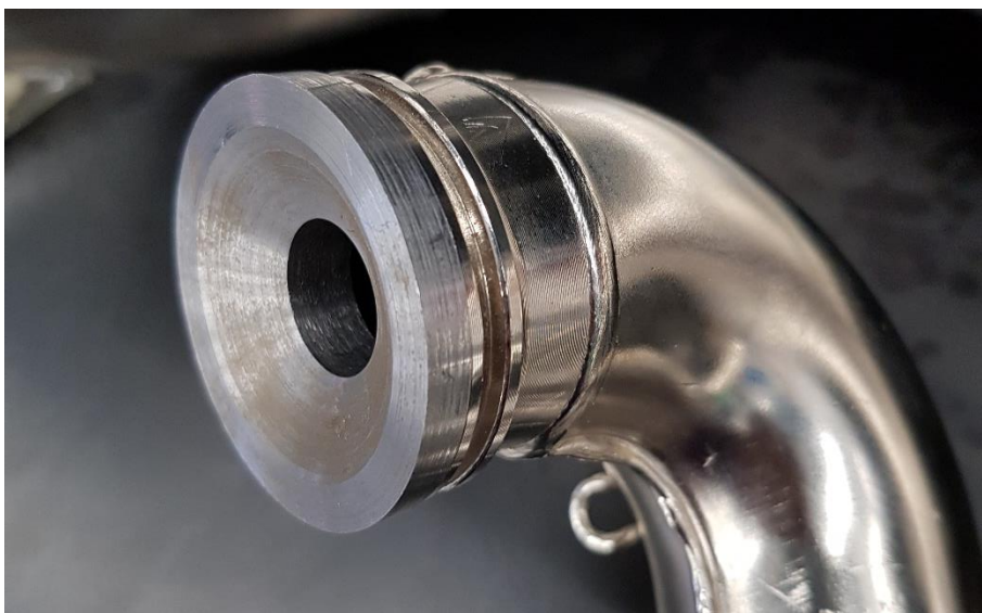
Figure 3 - Exhaust Port Restrictor Inserted in Modified Exhaust
