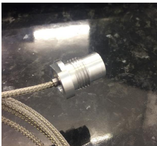
Figure 18 - Pressure Sensor in Insert
