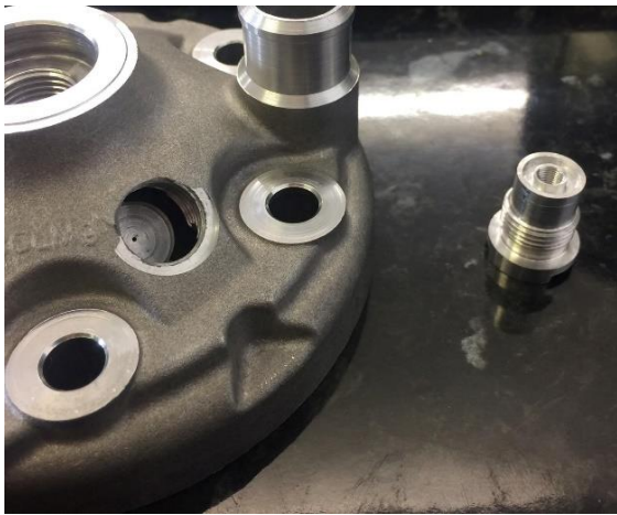
Figure 14 - Machined Head & Insert (GTPE, 2019)
