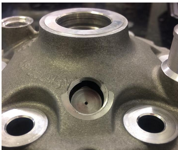
Figure 12 - Sealing Face and Outer Thread (GTPE, 2019)
