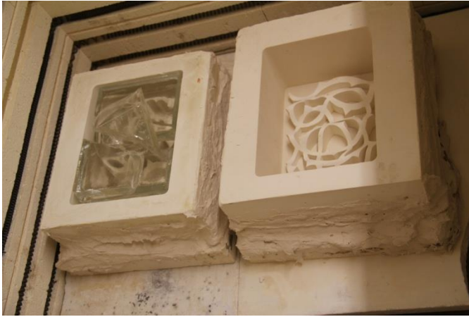
Figure 16. Moulds in preparation for kiln-firing
