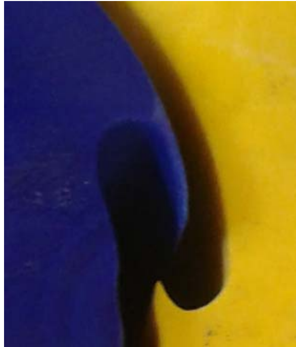
Figure 23. Example of material erosion cause by slow cutting speeds
