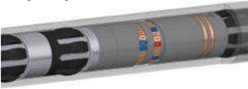
Figure 1 DefHi Eddy Current Probe Configuration
