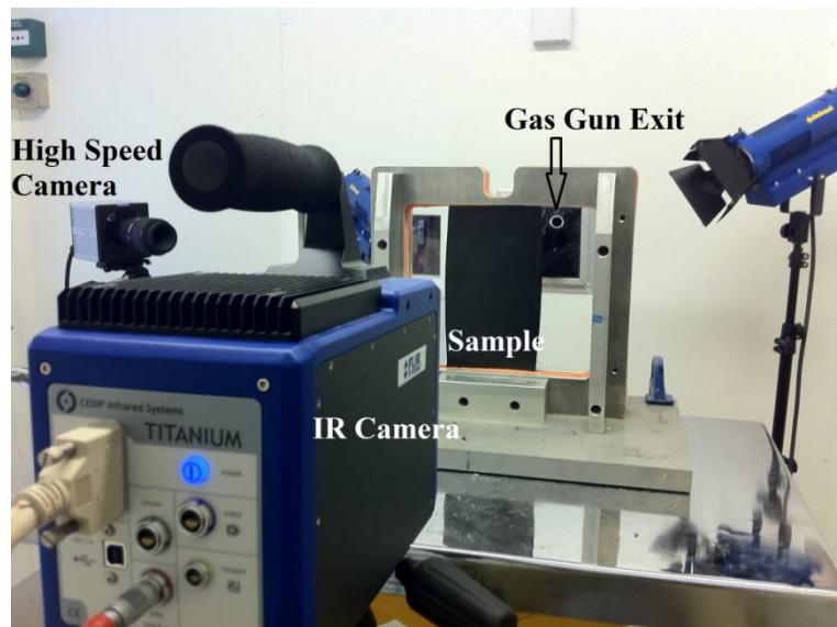
Figure 100 Experimental setup of gas-gun testing - view 1
