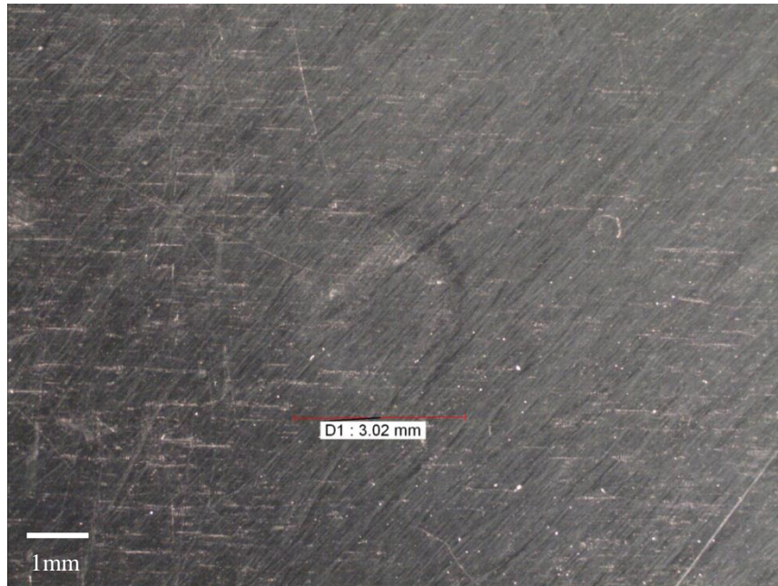
Figure 113 Microscopy image of 3QI16d8JC2 with damage dimensions
