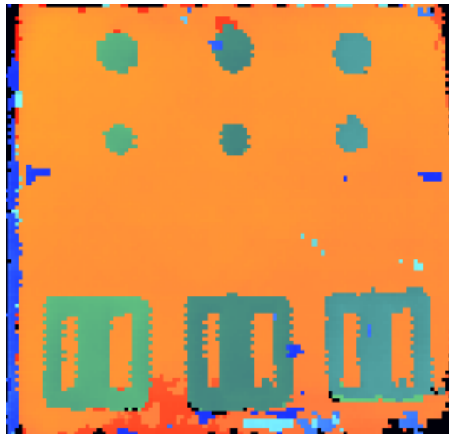
Figure 62 Time of flight (ToF) image for 9mm laminate (120×120mm) - Sample: 9TF1
