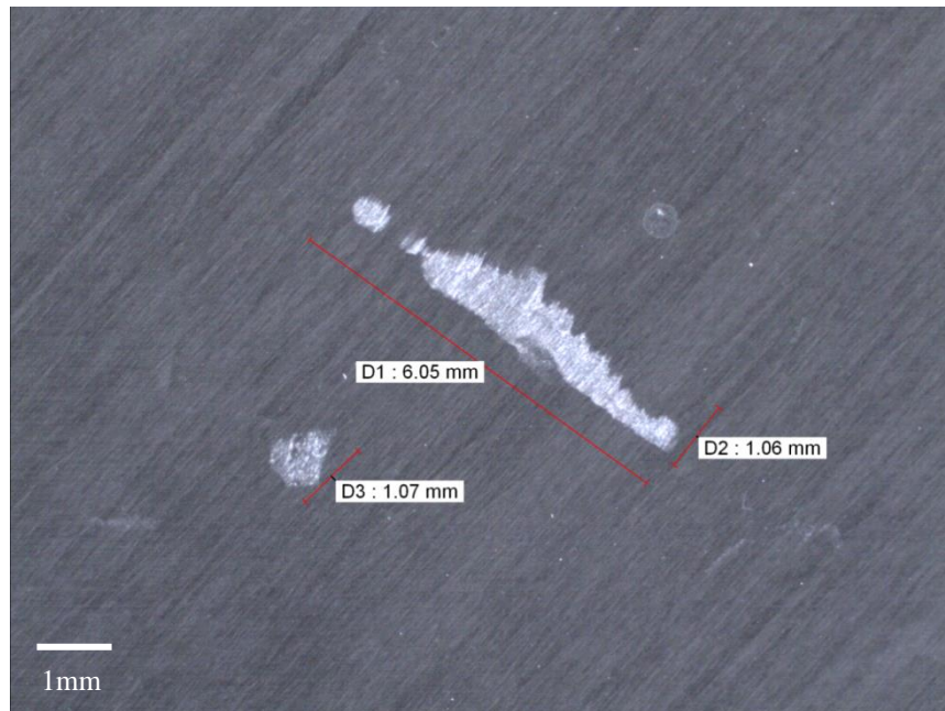
Figure 195 Microscopic image of 3TWI4.5JS3 laminate with damage measurements
