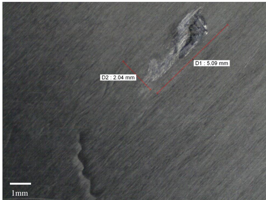
Figure 212 Microscope image of 6QI8JS1 with damage measurement
