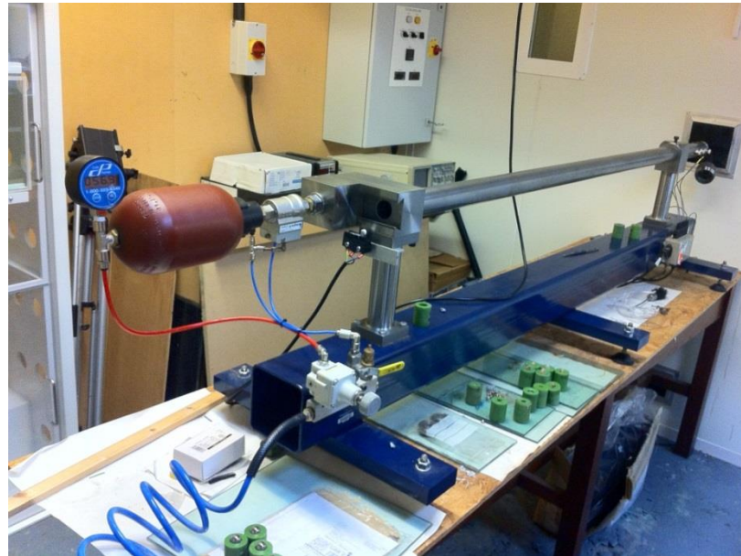
Figure 98 The Gas Gun - ballistic testing
