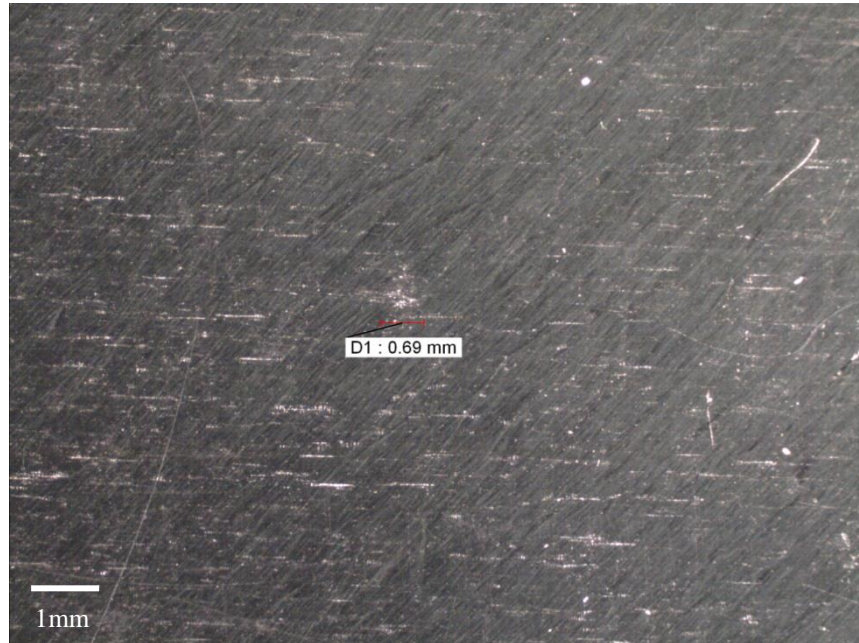
Figure 122 Microscopy image of 3QI12d4.5JC3 showing damage site – no visible damage
