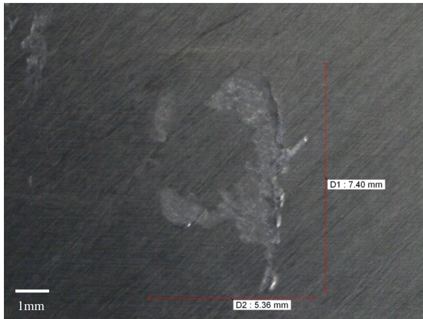
Figure 218 Microscope image of 6TWI12JS1 with damage measurements
