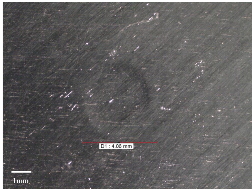
Figure 131 Microscopic image of 3TWI20d12JC3 with dimension of the damage
