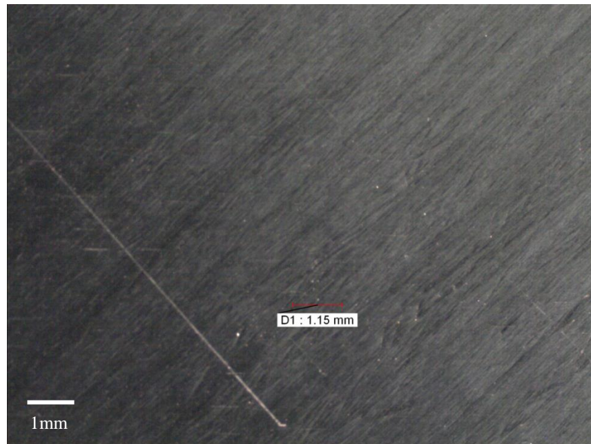
Figure 204 Microscopic image of 6QI20d12JC3 laminate with damage measurements
