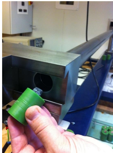
Figure 99 The gas-gun with sabot and stone
