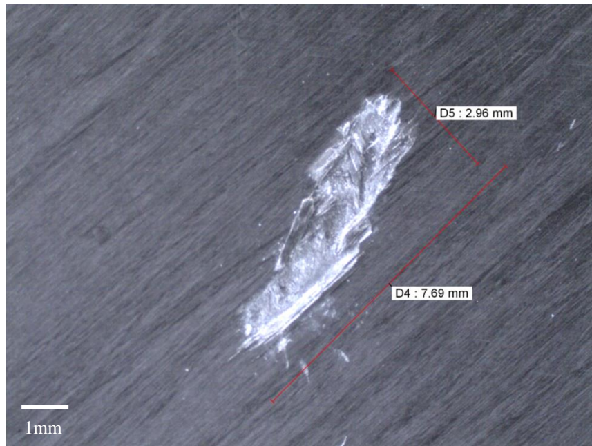
Figure 207 Microscopic image of 6QI12JS1 laminate showing damage area 1
