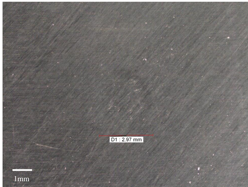
Figure 102 Sample: 3QI20d12JC2 - microscopic image with damage dimension
