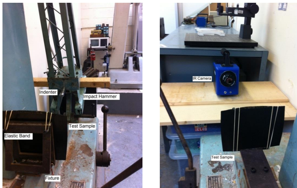
Figure 82 Indenter attached to the hammer on the left; and the infrared radiometer and test sample arrangement on the right
