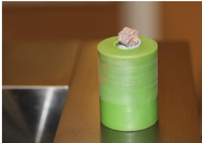
Figure 25 Sabot with stone that was introduced into the gas gun barrel for impact test
