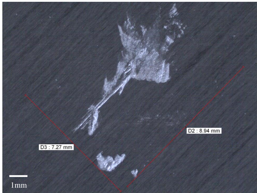
Figure 165 Microscopic image of 3QI8JS1 with dimensions of damage
