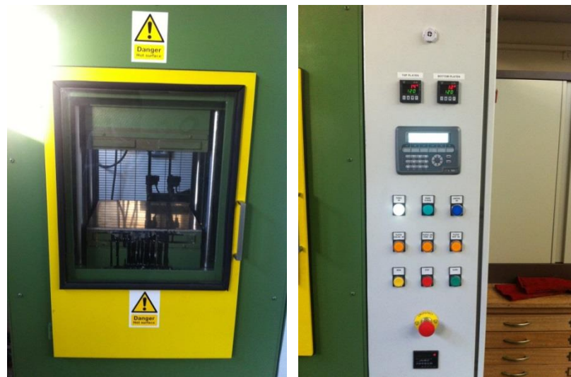
Figure 29 The hot plate (left) and the control unit (right)
