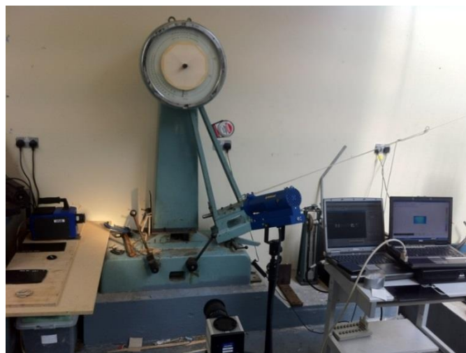
Figure 23 The modified Charpy impact test setup with infrared and high speed camera
