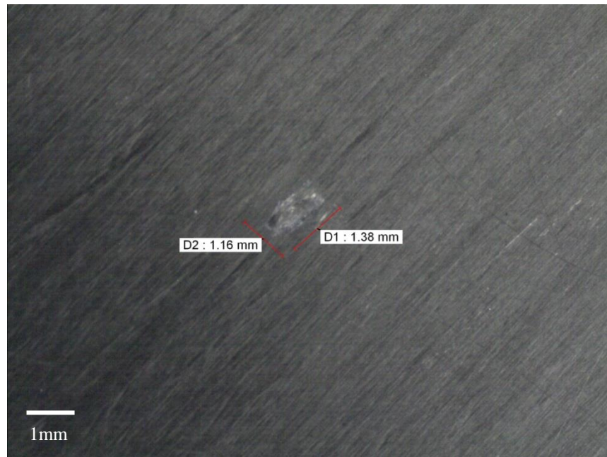
Figure 226 Microscope image of 6TWI4.5JS2 with damage measurements
