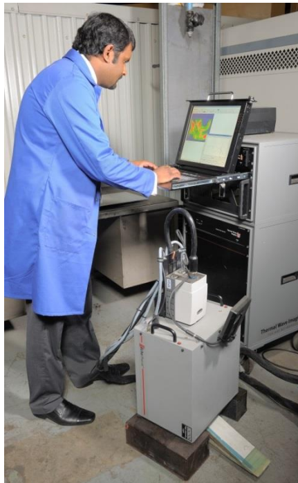
Figure 30 EchoTherm pulsed thermography system in use.
