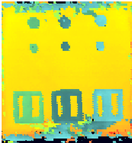
Figure 56 Time of flight (ToF) image for 3mm laminate (120×120mm) - Sample: 3TF1
