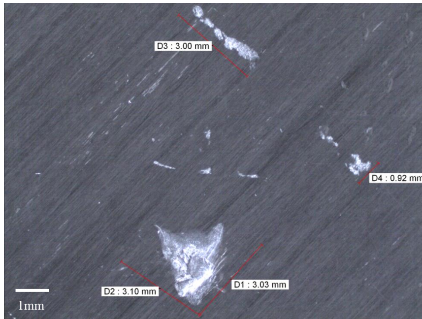
Figure 188 Microscopic image of 3TWI8JST1 laminate with damage measurements
