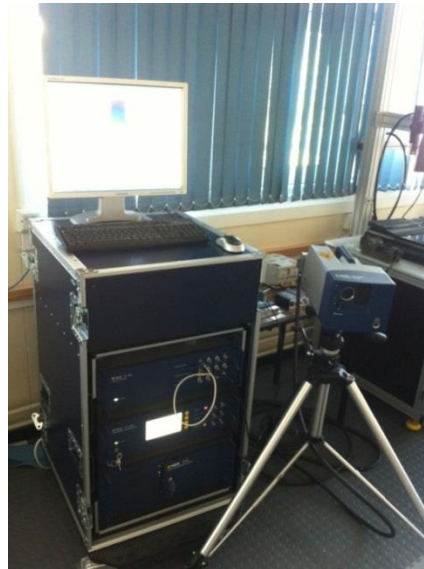
Figure 33 The Polytec PSV-400 laser doppler vibrometer
