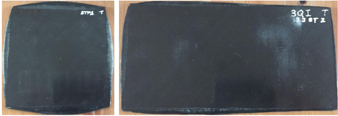
Figure 27 Representative parametric insert sample (120×120mm) (left) and impact sample (200×100mm) (right)
