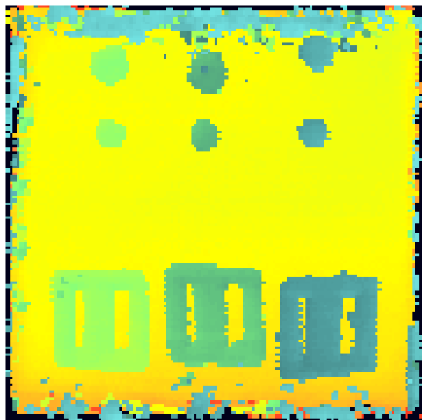
Figure 66 Time of flight (ToF) image for 3mm laminate (120×120mm) - Sample: 3BGF1
