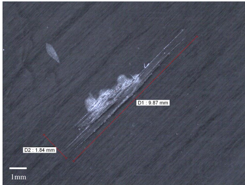
Figure 173 3QI4.5JS1 laminate's microscopic image with damage measurements
