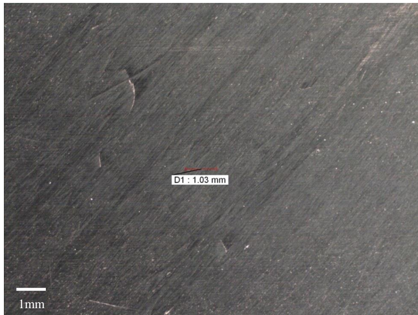
Figure 141 Microscopic image of 3TWI16d8JC2 with dimensions of damage
