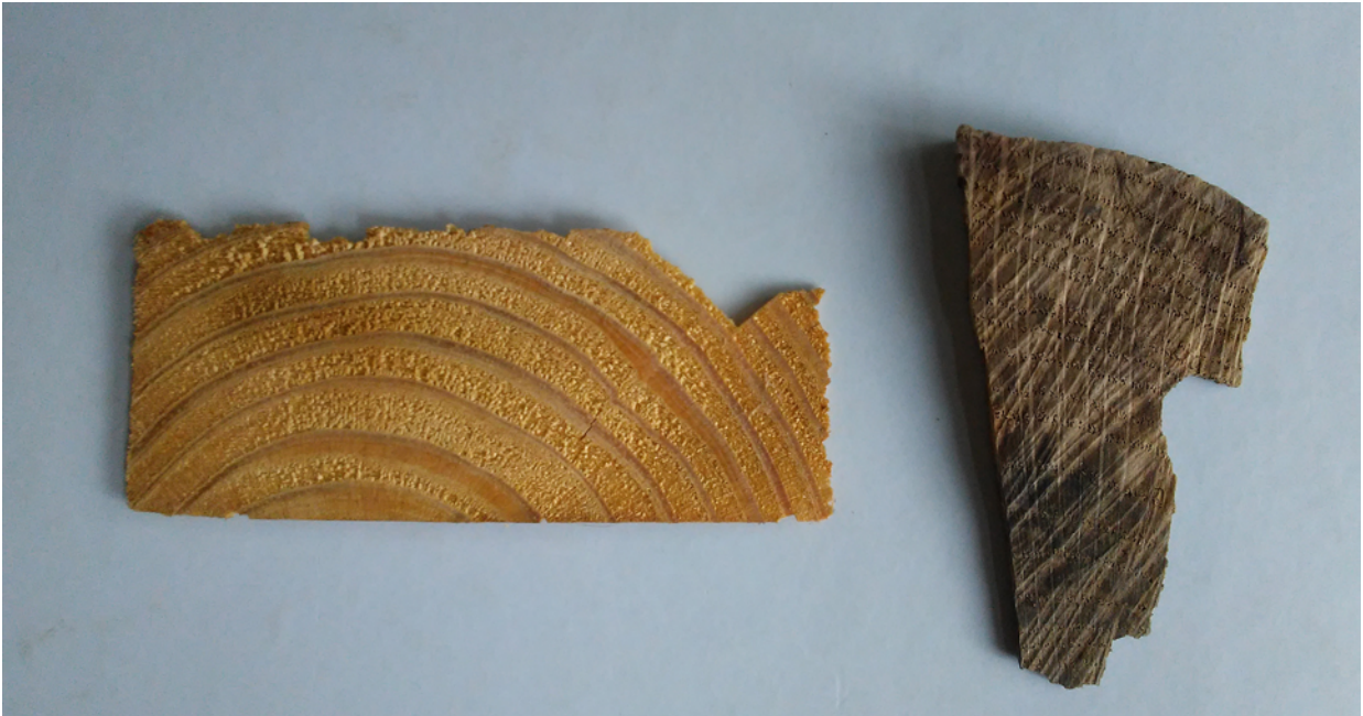
FIGURE 7. SLIVERS OF TRANSVERSE SECTIONS OF PINE ( PINUS SP.; LEFT) AND DECIDUOUS OAK ( QUERCUS SUBG. QUERCUS ; RIGHT), DEMONSTRATING THE VISIBLE DIFFERENTIATING FEATURES: COLOR, SHARPER DISTINCTIONS BETWEEN ANNUAL GROWTH RINGS IN PINE, POROUS EARLYWOOD IN OAK, AND MEDULLARY RAYS IN OAK. PHOTOGRAPH © SARA RICH, 2017.
