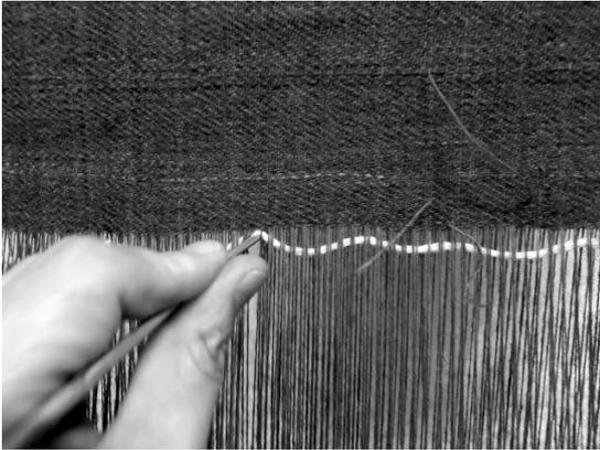
FIG. 3 A pin beater is used to position the weft. Detail of experimental weave at CTR, using white weft for illustration purposes.
