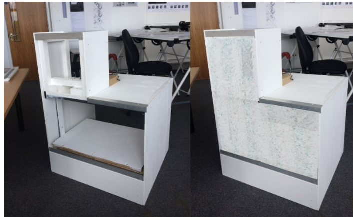
Figure 5, Full size carcass mock-up model made to hold the recycled glass panels, designed and made by the student
